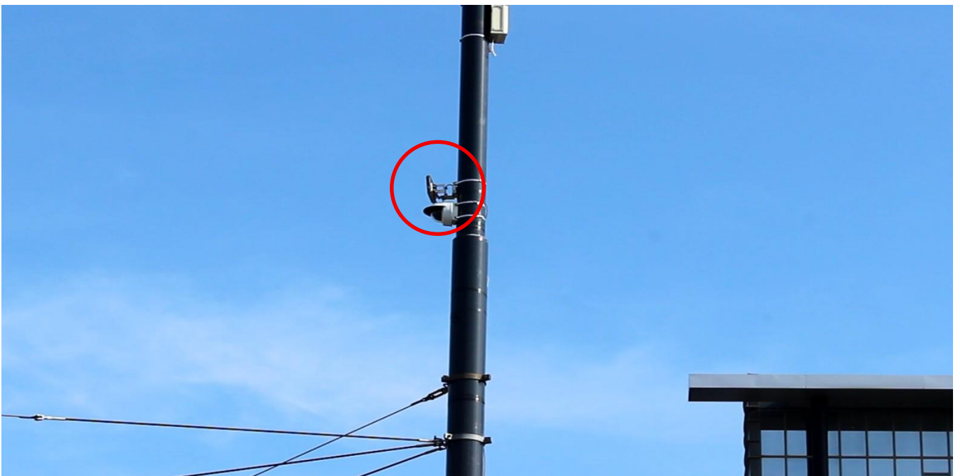
Figure 1: Roadside radar above a camera in the intersection between Mechelininkatu and Jätkäsaarenlaituri.
